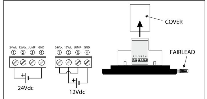
Fig. 1 Electric connection.
