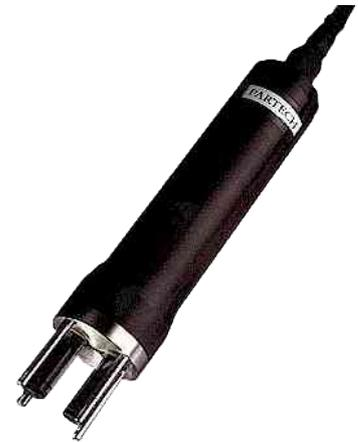
The Turbi-Tech 2000LS Sensor employs Infrared light at 860 nm using the 90° Light Scatter principle in accordance with ISO7027 (2000). The optics are housed in cylindrical glass tubes that are moved past a set of polyurethane wipers seals to carry out the cleaning process. The cleaning mechanism is then sealed by 2 Nitrile 'H' Rings that finish the cleaning process. The Nitrile seals can be exchanged for Viton if the process media dictates.
