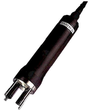
The Turbi-Tech 2000LA Sensor uses Infrared Light at 860 nm and operates using the Light Attenuation Principle. The optics are housed in cylindrical glass tubes that are moved past a set of polyurethane wipers seals to carry out the cleaning process. The cleaning mechanism is then sealed by 2 Nitrile 'H' Rings that finish the cleaning process. The Nitrile seals can be exchanged for Viton if the process media dictates.
